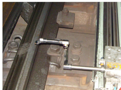
Fig. 3. Photo of rail coating system installed in Busan Metro Line 3.
