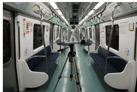
Fig. 1. Noise level measurement in the outdoor-tunnel and in the cabin of Busan Metro Line 3.
