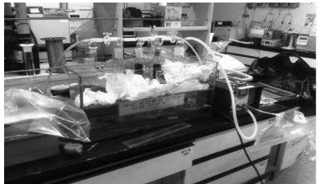
Fig. 3. Adsorption apparatus of Kapok fibers & Activated carbon.
